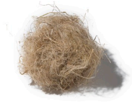
Loose long strand hemp bast. Different grades and lengths of fibre are available.
